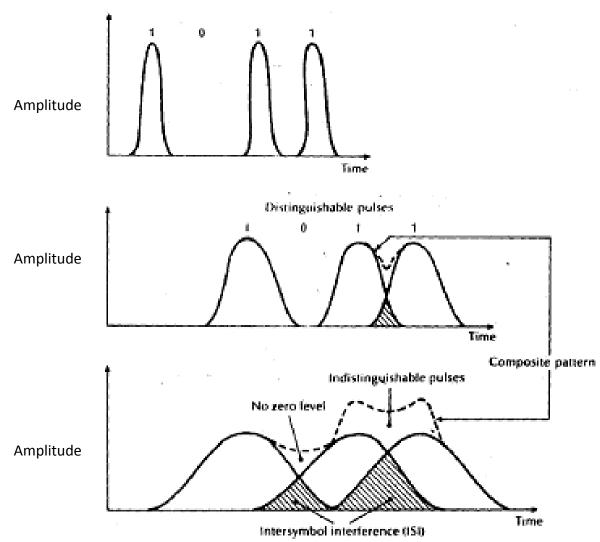
An illustration using the digital bit pattern 1011 of the broadening of light pulses as they are transmitted along a fiber: (a) fiber input; (b) fiber output at a distance L1;(c) fiber output at a distance L2> L1.
