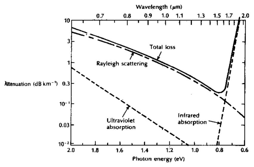
The attenuation spectra for the intrinsic loss mechanisms in pure GeO<sub>2</sub>SiO<sub>2</sub> glass
